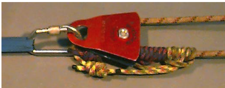
Figure 8 – Prusik minding pulley with fitted Prusik loops
