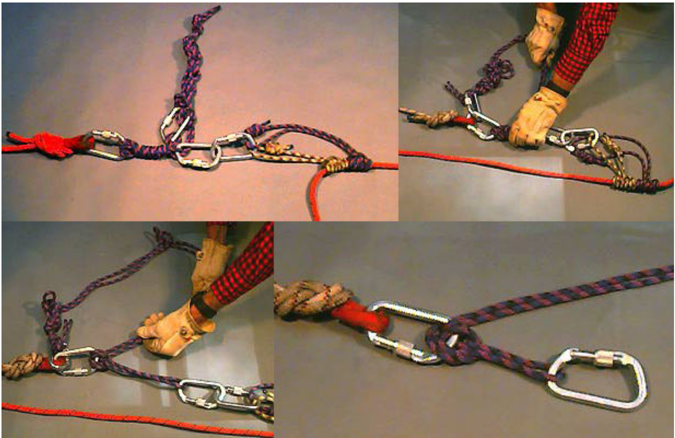
Figure 11 –Tandem Prusik belay attached to the belay line, load release hitch at the ready. (Top left) Starting to release tension with the load release hitch. (Top right) Load release hitch unwrapped, using the Italian hitch to release tension. (bottom left) The basis of the load release hitch, an Italian hitch. (Bottom right)
