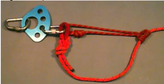
Figure 15 – Using a soft interface at the anchor.
