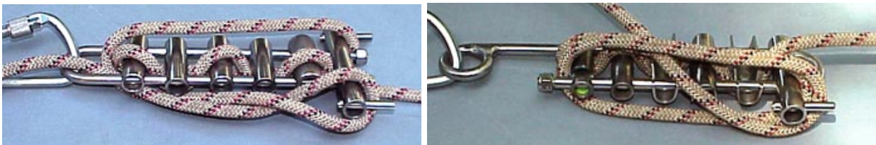
Figure 4 – Break bar racks, tied off.
