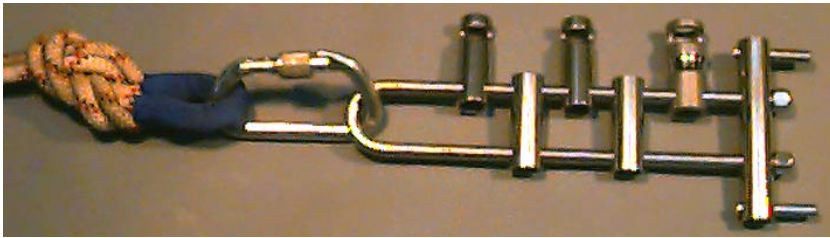
Figure 2 – Break bar rack, before rigging.
